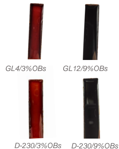
Successful replacement (increase of mechanical properties) of Jeffamine curing agent up to 6 wt.% by OBs lignin
