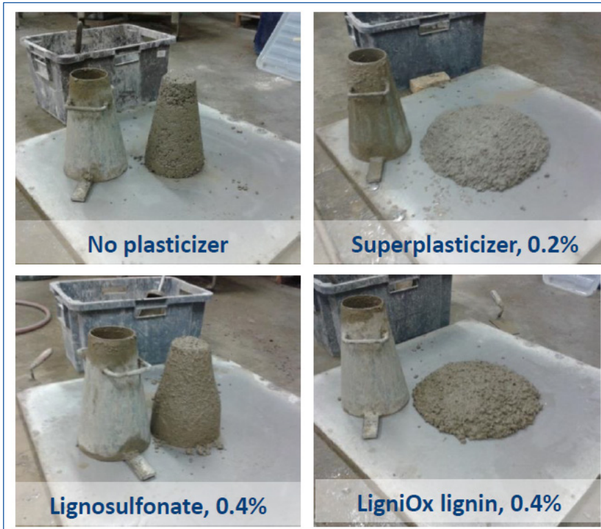
Figure 3. 5 Performance of the lignin-based superplasticizer LigniOX
